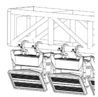
Two quarter-turn brackets are supplied with the fixture if it is to be flown above the ground. Rig the fixture to a support truss or structure using the supplied brackets and suitable clamps.
