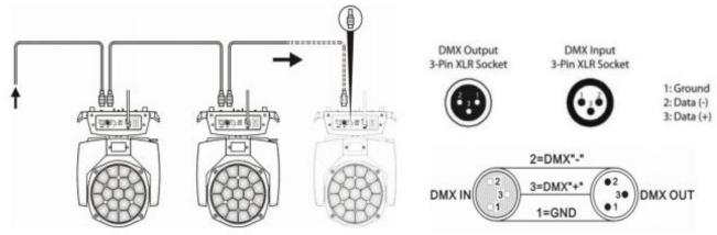
For installations where the DMX cable has to run a long distance or is in an electrically noisy environment, such as in a discotheque, it is recommended to use a DMX terminator. This helps in preventing corruption of the digital control signal by electrical noise. The DMX terminator is simply an XLR plug with a 120  $\Omega$  resistor connected between pins 2 and 3, which is then plugged into the output XLR socket of the last fixture in the chain. Please see illustrations below
