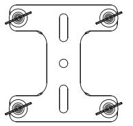
In this case the fixture can hang on the truss in horizontal position only, not sideways .
