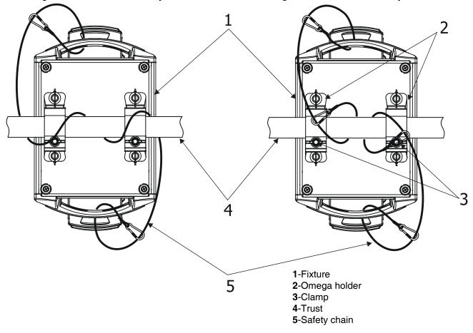
The fixture can be also rigged by means of the mounting adapter (option) for one Omega holder:.
