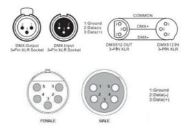
For installations where the DMX cable has to run a long distance or is in an electrically noisy enviroment, such as in a discotheque, it is recommended to use a DMX terminator. This helps in preventing corruption of the digital control signal by electrical noise. The DMX terminator is simply an XLR plug with a 120  $\Omega$  resistor connected between pins 2 and 3, which is then plugged into the output XLR socket of the last fixture in the chain. Please see illustrations below.
