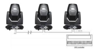
Connect the DMX-output of the first fixture in the DMX-chain with the DMX-input of the next fixture. Always connect one output with the input of the next fixture until all fixtures are connected. Up to 32 fixtures can be connected.
